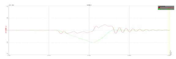
(2) Test once with the rated speed 0.50 m/s, rated load 750 kg, system mass 2350 kg.
